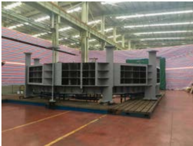
Figure 2: Assembled Stator Frame for Karuma
