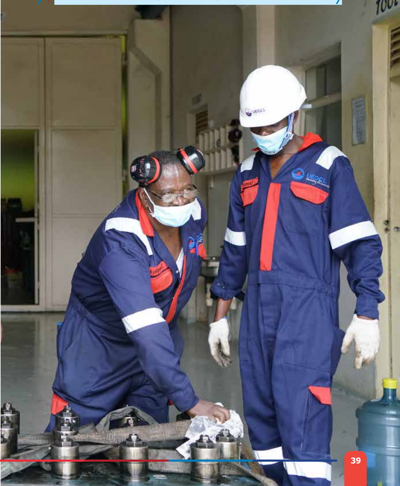
UEGCL operations and maintenance staff at Namanve Thermal Power Plant cleaning one of the fuel injection valves.
